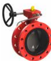
Series 75 Butterfly valve Centric with fixed liner Double flanged short DN50-300 PN10/16 Ductile iron FM approved
