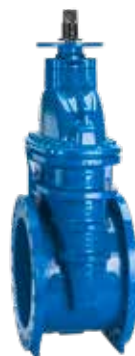
Series 55 Flanged gate valve with post indicator flange DN450-600 13.7 bar (200 PSI), UL/ULC listed 17.2 bar (250 PSI), FM approved PN16 drilling 316 stem Ductile iron
