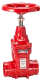
Series 06/37 Grooved end gate valve with position indicator DN50-300 PN16 drilling Ductile iron VdS approved (DN50-200 only)
