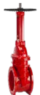
Series 55 Flanged gate valve with rising stem OS&Y DN450-600 13.7 bar (200 PSI), UL/ULC listed 17.2 bar (250 PSI), FM approved PN16 drilling 316 stem Ductile iron
